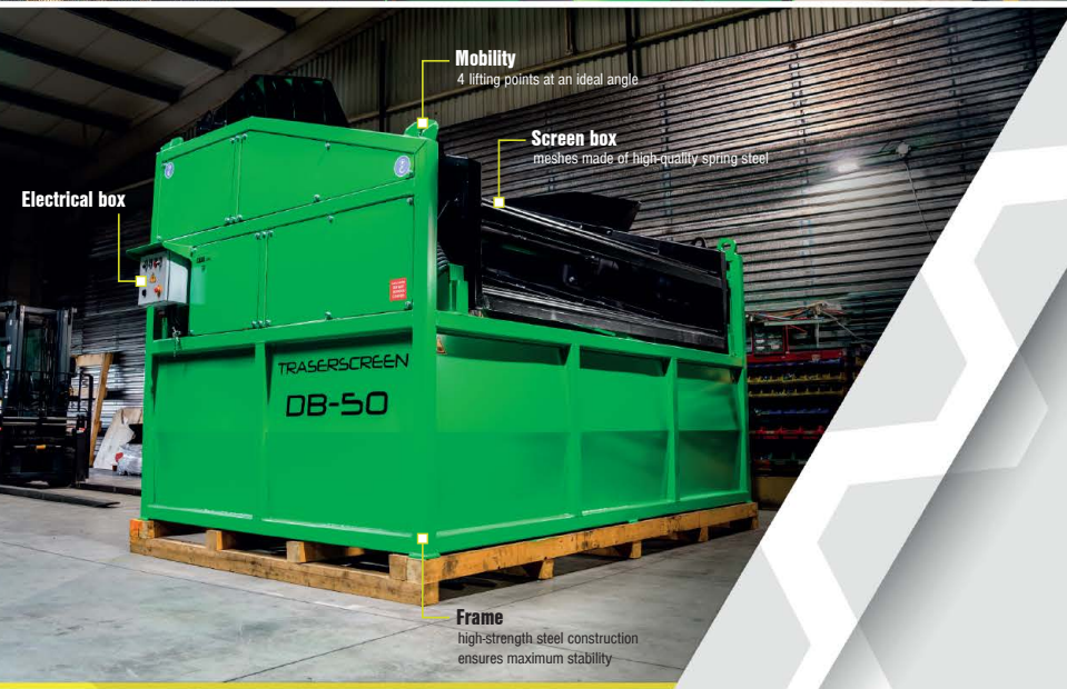
Screen box on 12 steel springs
